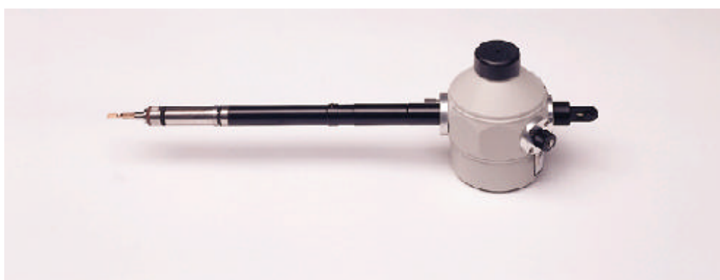
Fig. 2.1 – An LN 2 cooled TEM sample holder from Gatan Inc. The dewar to be filled with the liquid nitrogen is visible on the right. The thermal isolation is obtained by evacuating through a zeolite pump the space between the outer and the inner walls of the dewar.
