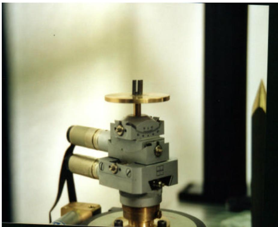
**Figure 2.3:** *The picture shows the Si channel-cut monochromator*
